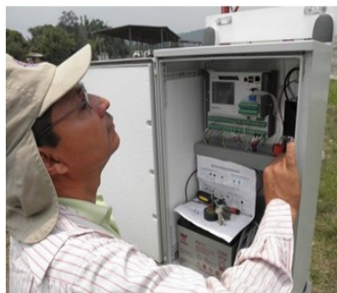
The project is helping to acquire, calibrate and install automatic weather stations to identify and prepare for future extreme weather events. Photo: UNDP Honduras
