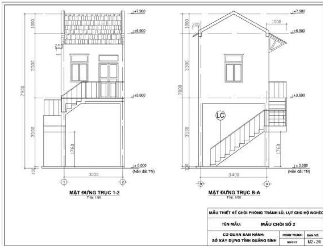
Figure 8: Design Specifications for improved housing designs
