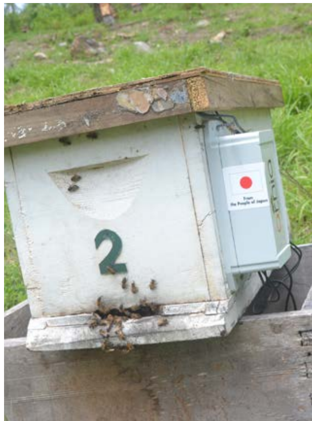
Monitoring system installed on a bee hive to track humidity, temperature and acoustics
