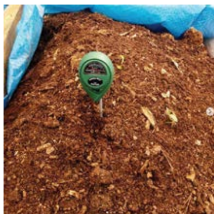
Soil and pH monitor being used by a Dominican farmer to test optimal conditions for planting
