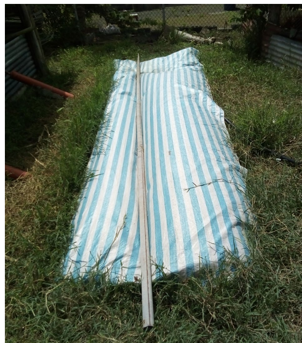
Pictured above is a large component of a biodigester system which uses a bag to allow for an easier installation process.
